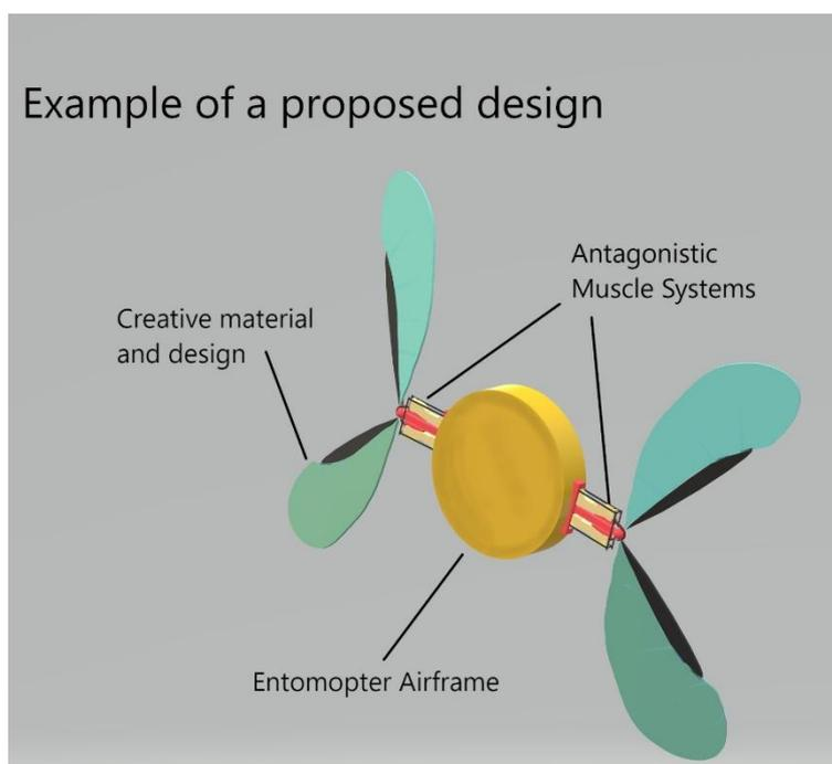
**Figure 3:** Graphic design of an example of structure that may be prototyped for purposes of this study.
