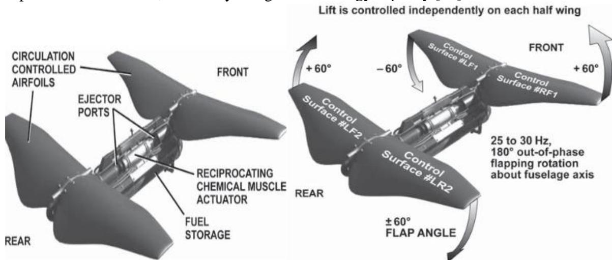
**Figure 4:** Schematic of the proposed design by Michelson [25]. The antiphase flapping and non-fixed wing stroke resemble insect flight mechanisms, allowing for motion in 3 degrees of freedom.
