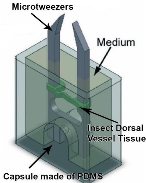
**Figure 1:** Micro-tweezers being packaged in medium, in a capsule made of PDMS, submerging the Insect DVTs. The gap between the capsule and the medium is filled with parylene materials which prevents the medium from evaporating [14].
