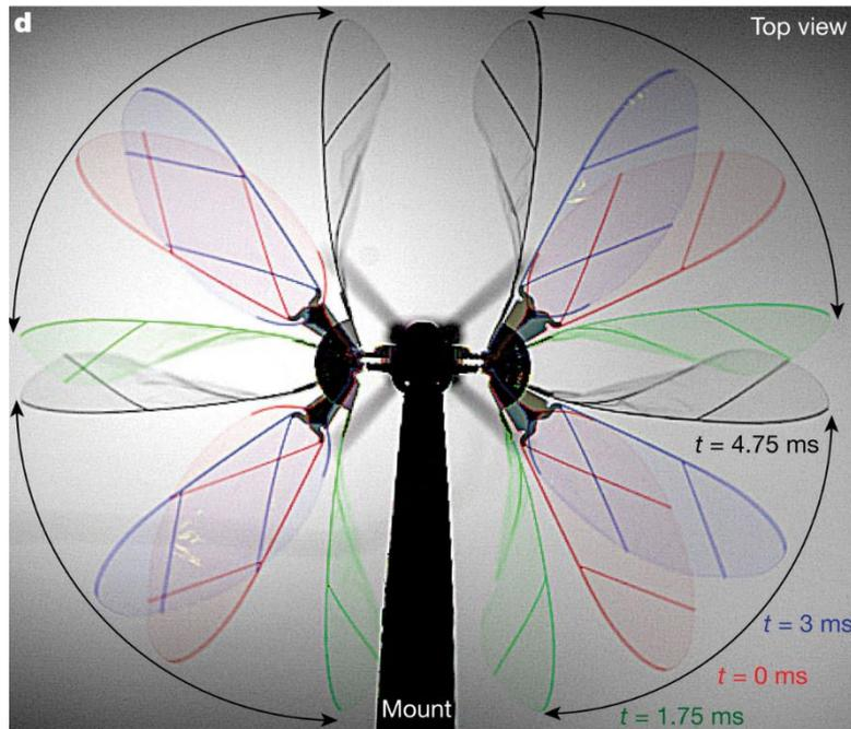
**Figure 5:** Example of an entomopter, the RoboBee also employs 2 sets of wings. This provides a small physical profile [24].
